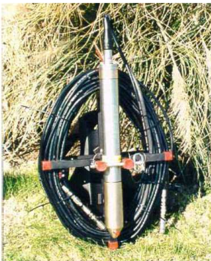
DHS-5500 Downhole Source
