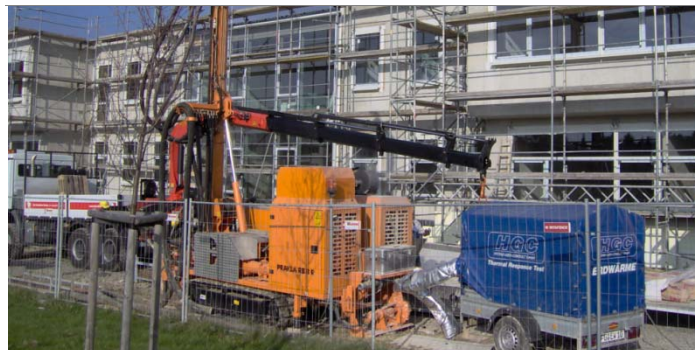
Thermal Response Test to determine ground parameters
