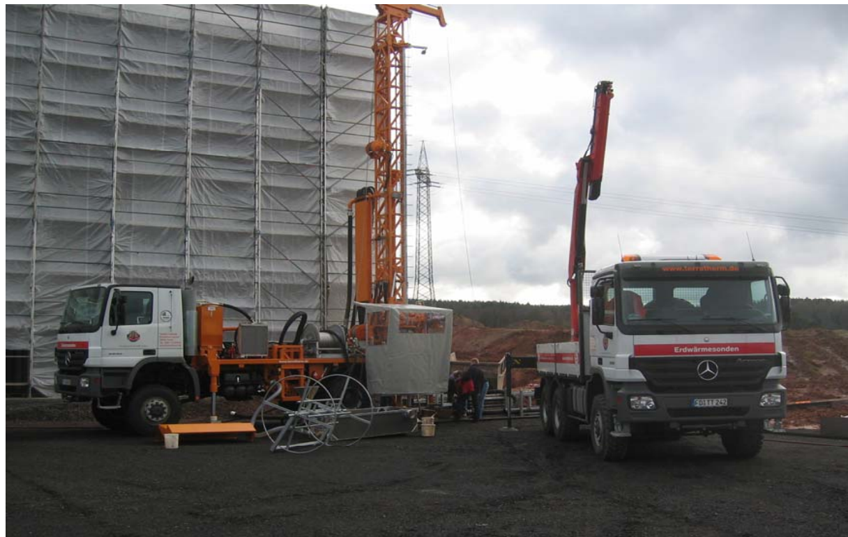
Mobile drilling rig Bauer-Prakla RB 30 GT
