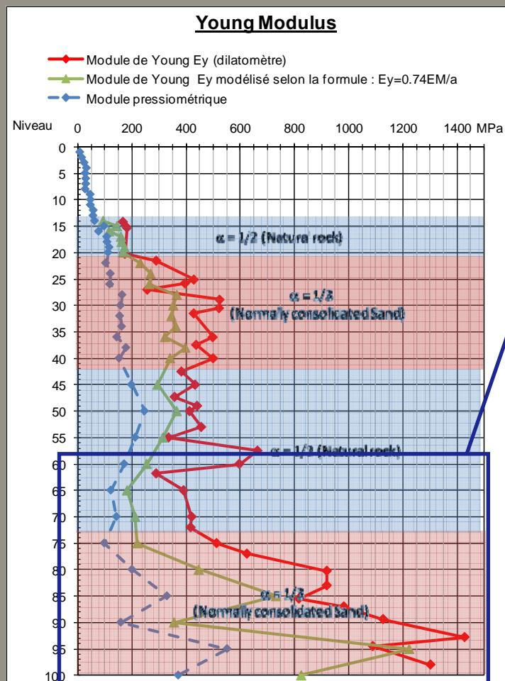
Significant difference between Young's modulus measured by the dilatometer tests and Young's modulus deducted by the pressuremeter tests :
