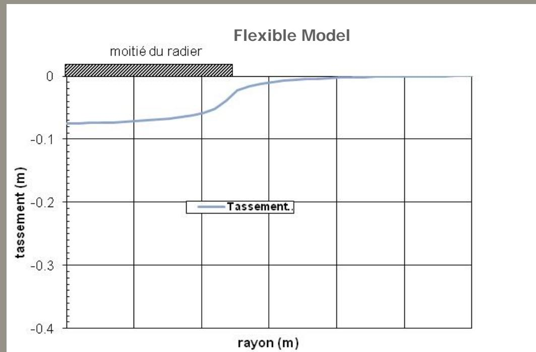
Estimation of settlement with load uniformly distributed over the raft of 6.3 Bar, is equal to 7.8 cm at the center of the raft
