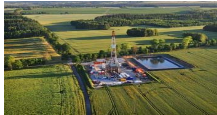
Pad during drilling (1 year)
