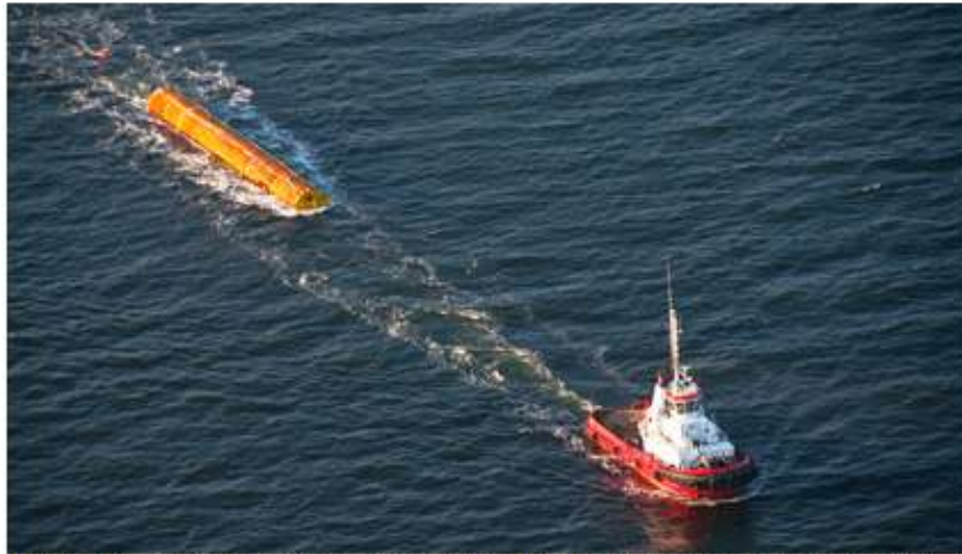
Turbine foundation on its way to Anholt Offshore Wind Farm. Photo: DONG Energy.
