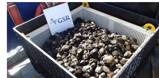
A batch of polymetallic nodules, just after recovery
